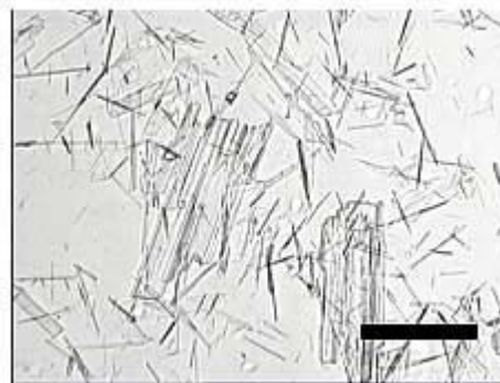
Figure 6. Microscopy picture of \beta -sitosterol suspension recrystallized containing 1% (wt/wt) Polysorbate 80 with a stirring time of 30 seconds. The picture was taken 1 day after preparation (bar = 100\ \mu\text{m} ).
